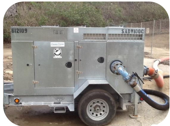
Water Pump with Noise Insulation
