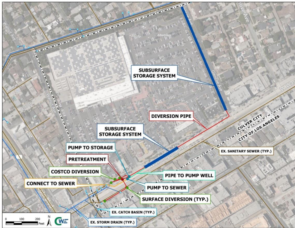
Figure 2-2 Subsurface Storage System Approach
