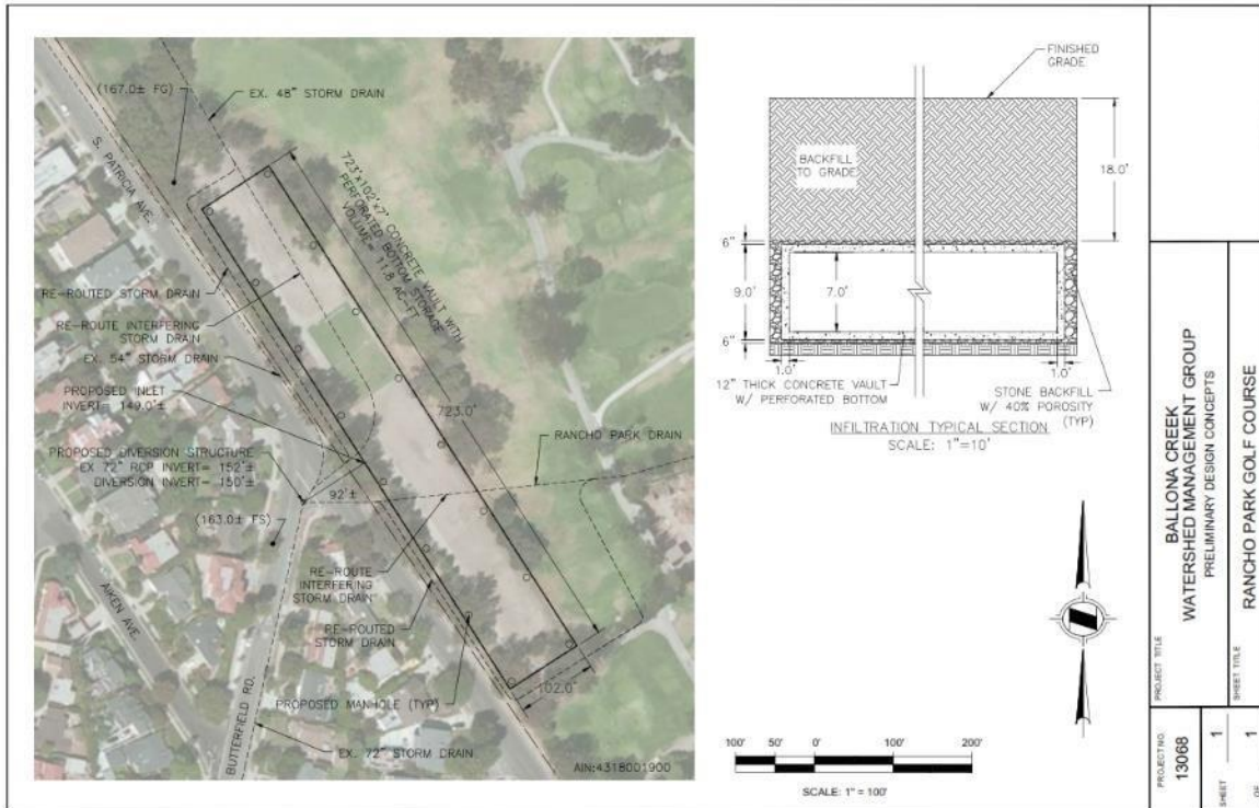
Figure 4-7 Rancho Park Golf Course and Cheviot Hills Recreation Center Surface and Subsurface Infiltration Basin – Preliminary Design Concepts
